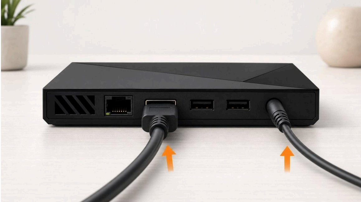
Back of the NVIDIA Shield Pro showing the HDMI and power connections
