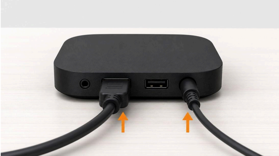
Back of the Xiaomi TV Box S showing the HDMI and power connections
